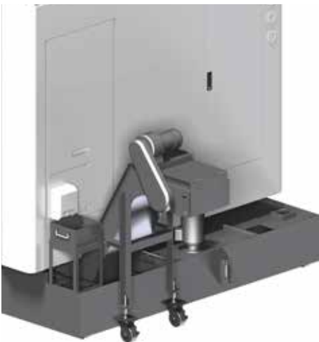
Coolant tank capacity 260 L (80% full)
