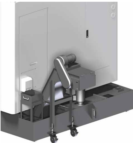
Coolant tank capacity 400 L (80% full)
